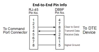
RJ-45 connector plugs into Command Port of MultiVOIP GSM.
